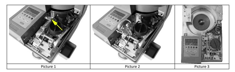
Pull the metal plate marked on picture 1 and lift up the mechanism (picture 2). With a soft brush or cloth you can remove the coarse dust deposits from the transport area of the coins. If you have jammed coins, you also have access to the corresponding area to remove the coins.
